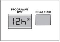
To activate the delay timer, press the START PAUSE button. The amount of time remaining until the programme is set to start is continuously displayed (e.g. 15h, 14h, 13h, ... 30' etc).
